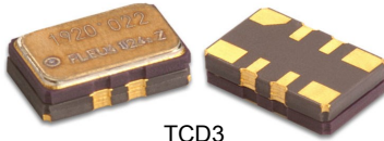
TCD3 3.2 x 5.0 x 1.50 mm LCC Ceramic Package
