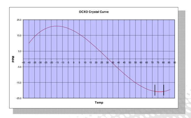
The crystals for these oscillators are manufactured so the upper turning point is above the highest specified temperature range. The crystal and associated circuitry is heated to and maintains a narrow temperature window around that point on the crystal, and the device is tuned to frequency at that temperature.
