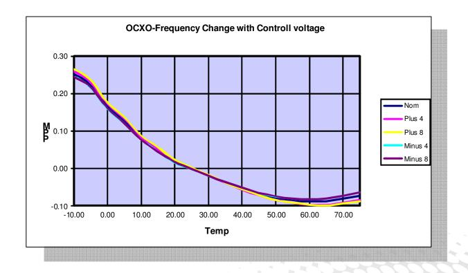
The OCXO has the added advantage of exercising the crystal over a very narrow temperature window, typically a couple degrees or less. This greatly reduces the chances of exciting unwanted modes in the crystal. The greatest drawbacks to this approach are the size of the devices and the power requirements. As technology moves forward, both the size and power requirements of these devices continues to decrease.
