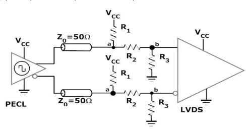
There is not an exact solution for 3.3V. Here are optimum values to use: for 2.5V the schematic must change, move R1 from VCC to 'b' and move R3 from 'a' to ground.
