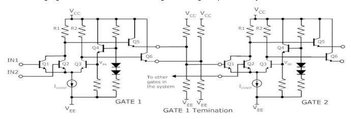
It is important that both outputs are terminated for best performance. If only one output is used, the duty cycle and iitter can be adversely affected.
