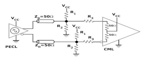
The  $V_{CM}$  of the CML input and the signal swing on the CML input will need to use the minimum levels allowed. The CML input is reduced to about 0.125V PP which is still within the CML input minimum level specification. Therefore R3 is 275 ohms.
