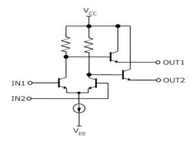
It must also be noted that the LVPECL differential input requires a common mode reference voltage. This voltage is nominally Vcc – 2.0V. For 3.3v LVPECL, this common mode reference supply is 1.3v. Extra power supplies are not attractive so alternative termination schemes will be shown.
